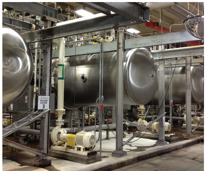
Polish filters in our Trenton Brewery show one step of many in the brewing process, where we are able to capitalize on energy and water efficiencies.
