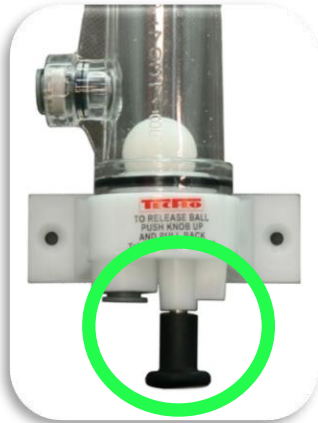
Figure 9 - Fob plunger pushed up (Cleaning Only)
